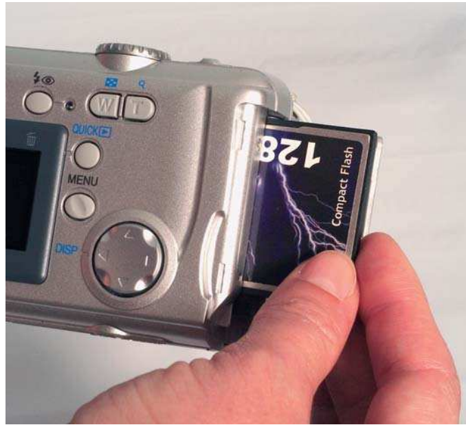
Figure B.2 The memory cards are inserted into the camera via an access flap so that full cards can be replaced with empty ones.
